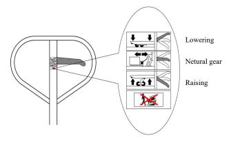
The control handle knob has three positions (up, middle, down). Up Push the control handle knob to the lower position, then bob up and down the handle to lift goods on fork.
